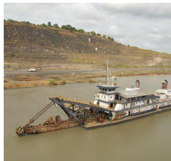
Fig. 11. A floating suction dredger in front of the West Culebra Slide in 2012, with its suction pipe and rotating head raised out of the water while not in action.
