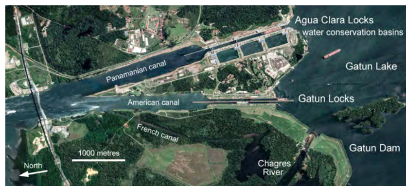
Fig. 15. Old and new locks out of Gatun Lake at the Atlantic end of the Panama Canal. The Earth components of the Gatun Dam are the entire areas covered in paler green grass, with the curved crest of its concrete spillway at the centre above the Chagres River. (Base images from GoogleEarth.)
